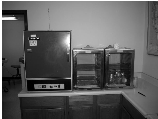
Figure 9 —Chapter 5, Seed Testing: a convection oven and desiccator are used to conduct a seed moisture test.
