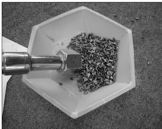
Figure 3 —Chapter 5, Seed Testing: the seed probe is emptied by pouring the seeds out the top.
