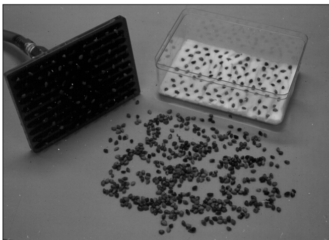
Figure 17 —Chapter 5, Seed Testing: a vacuum counter is often used to count out seeds for weight determinations and for planting germination tests
