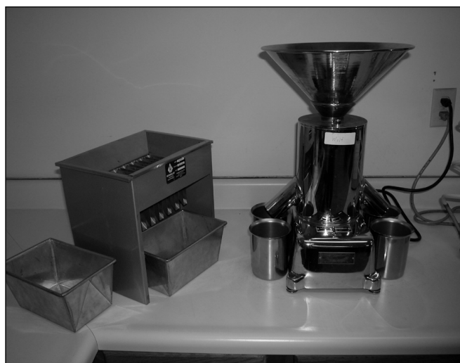
Figure 7 —Chapter 5, Seed Testing: a soil divider ( left ) and a gamet divider ( right ), devices that systematically mix and divide seed samples.
